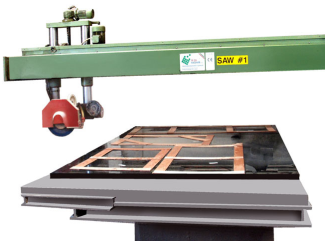
Example of template arrangement before cutting the slab.
